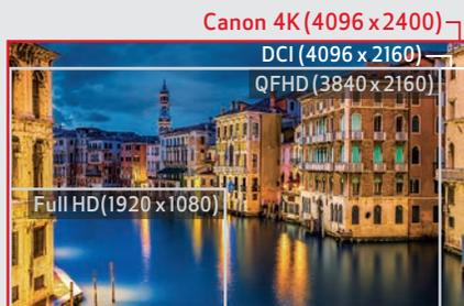
At 4096 x 2400, Canon's 4K resolution generates a bigger, richer picture made up of more than 9.8 million pixels – higher than the Digital Cinema Initiative (DCI) standard for 4K cinema (4096 x 2160) and more than QFHD (3840 x 2160), the resolution standard for 4K TV.
